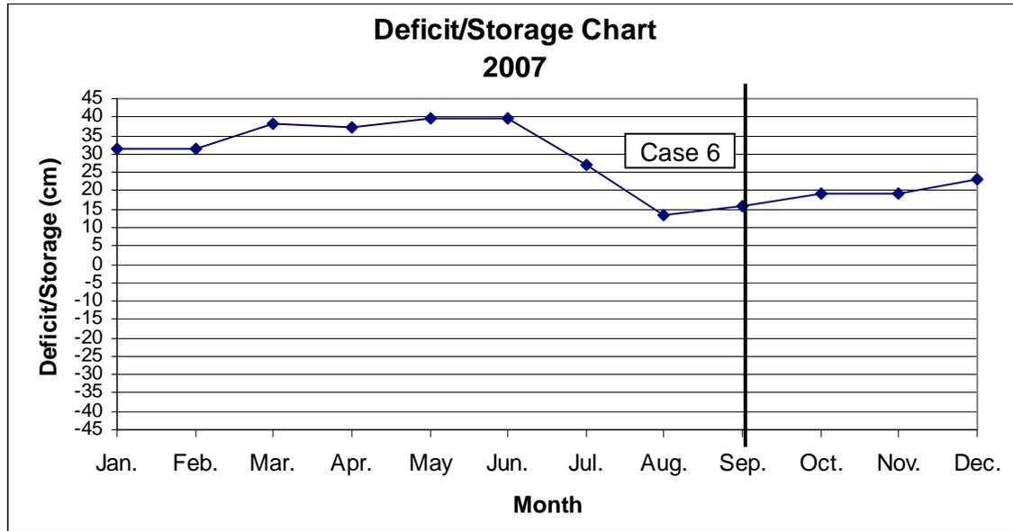
Figure 9. Moisture Storage/Deficit Profile for Case Study 6.
