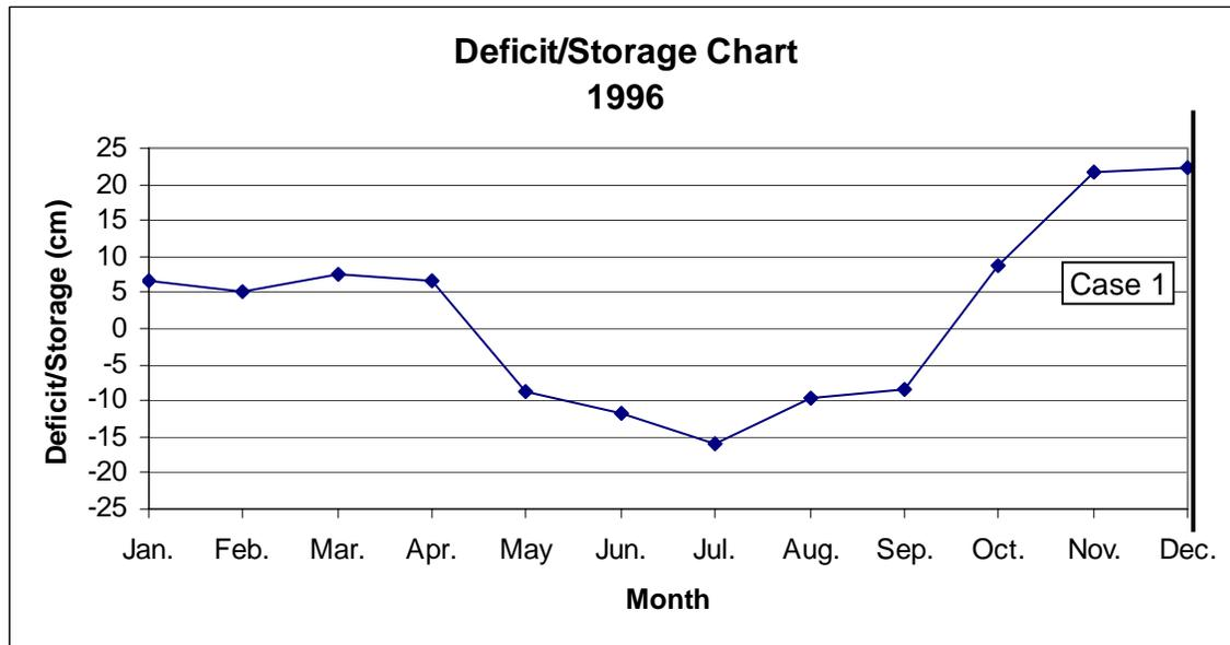
Figure 2. Plot of calculated deficit or storage values in cm for 1996. The vertical line on the right side indicates the approximate sampling date for Case Study 1.
