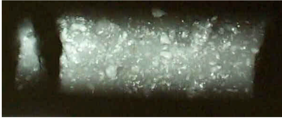
Fig. 7 X-ray of soil sample obtained from utility trench (location shown in Fig. 5). Note the soil clods within sample.
