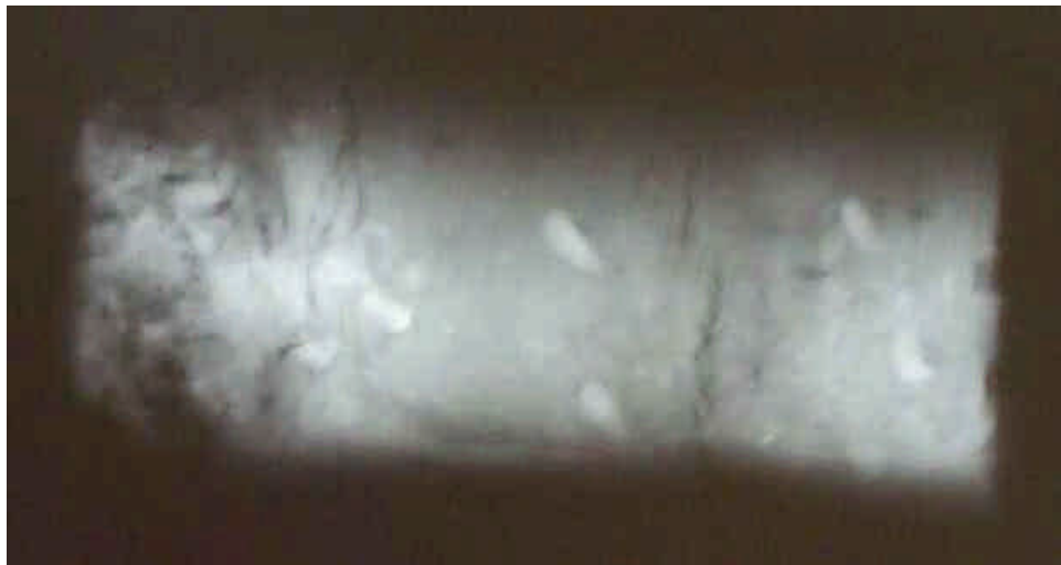
Fig. 8 X-ray of sandy clay fill placed at above optimum moisture content. Note relatively fewer soil clods compared to sample in Fig. 7.
