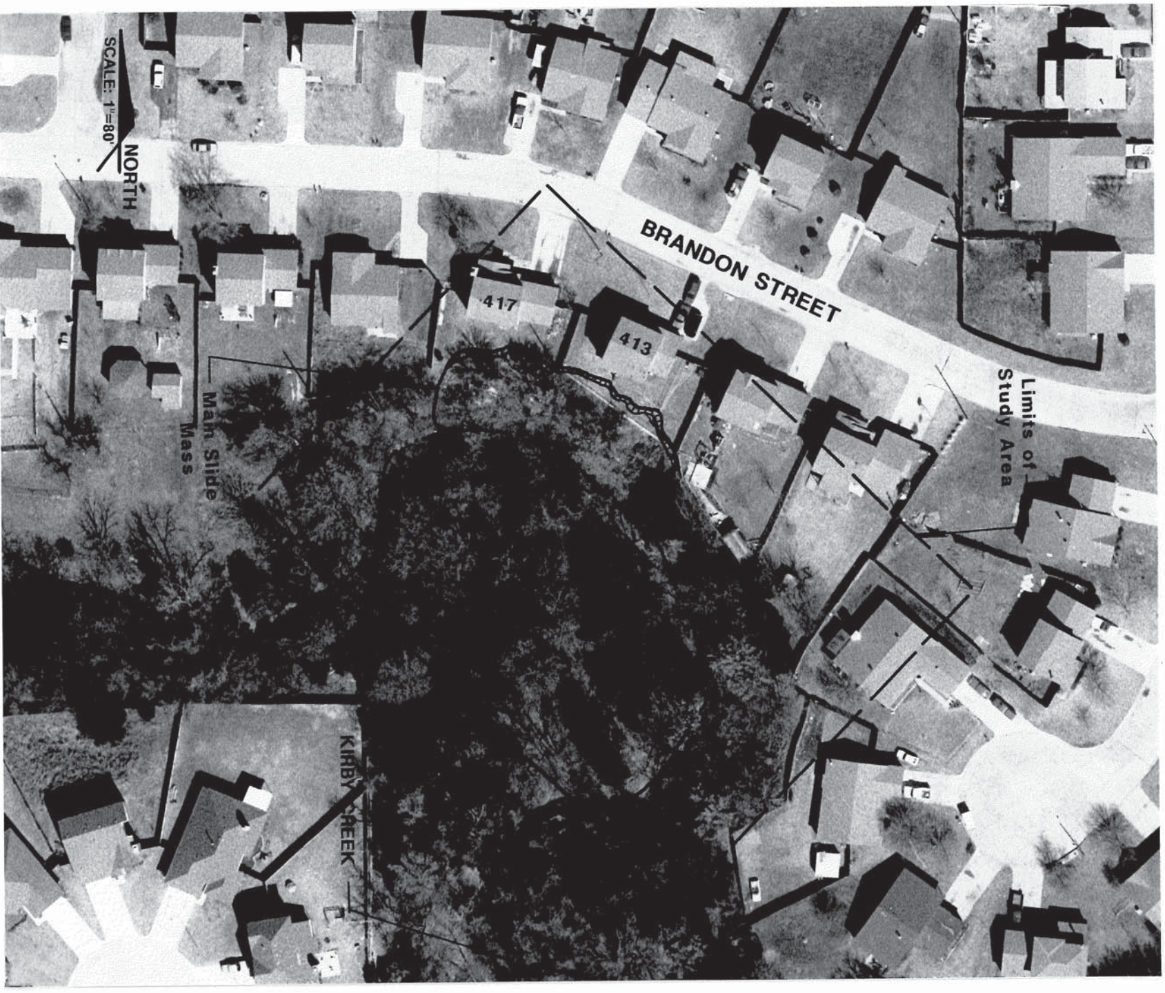
Photograph 10. Aerial view of residences and creek prior to slope failure. Note proximity of rear yards to creek bank.
